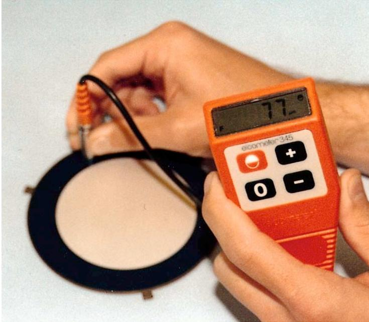
ESL insulating dielectrics are screen printed onto the appropriate steel using 165 mesh stainless steel screens with 0 $\mu$ m emulsion. Each fired layer should be 25-30 $\mu$ m thick. Measurement is carried out using a coating thickness gauge (e.g. Elcometer 345 is shown in the picture).
